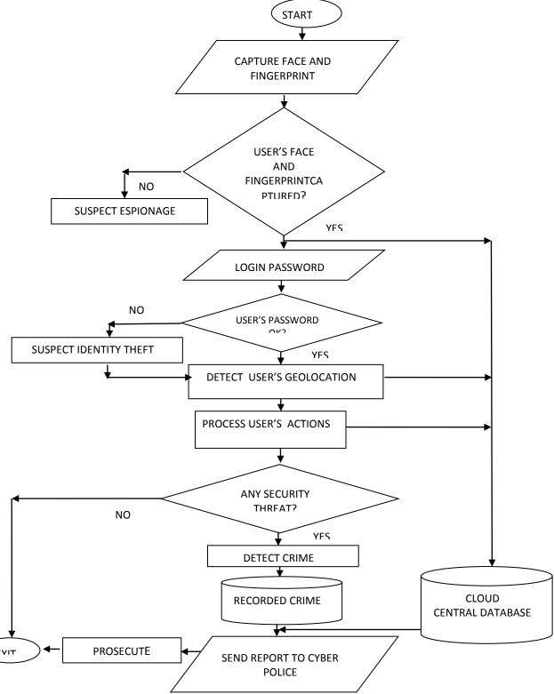
Figure 5. System Flowchart of the Enhanced Cyber Crime Prosecution Information System
