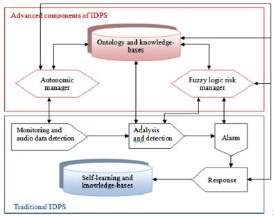
Figure 1. A Typical Intrusion Detection System [15]
