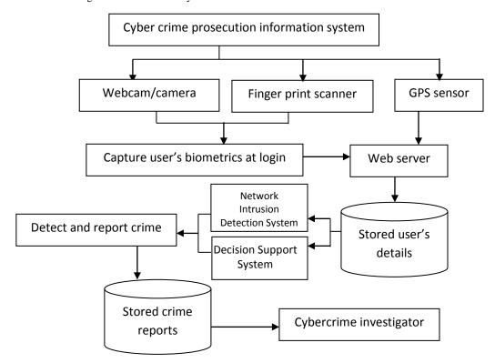
Figure 6: High Level Model of the Enhance Cyber Crime Prosecution Information System
