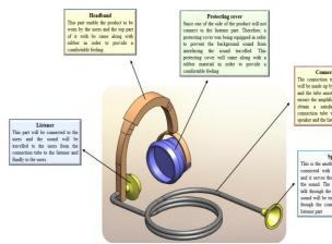
Figure 4: Concept 3 - modified wearable speaking tube
