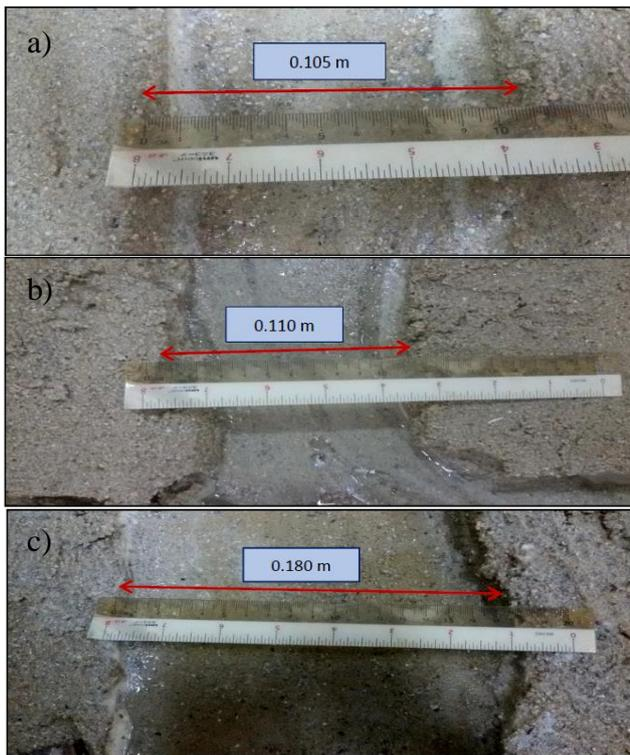
Fig. 4: Lateral movement  $W$  when flow rate  $Q$  is 0.36 L/s at (a)  $\beta$  is 60 degree, (b)  $\beta$  is 80 degree and (c)  $\beta$  is 90 degree
