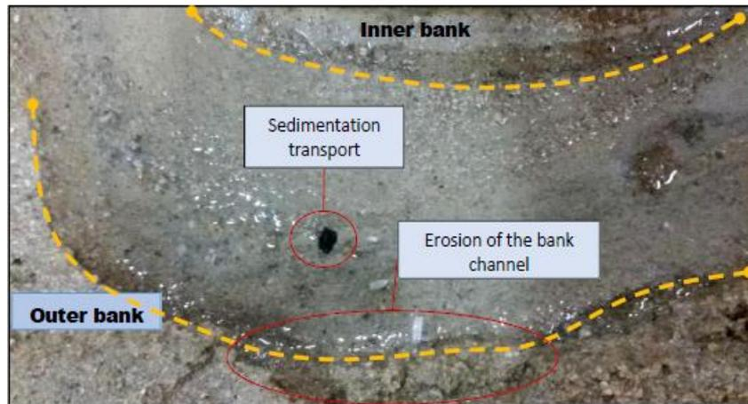
Fig. 3: Erosion at the bank channel of  $M_3$  with angle of direction  $\beta$  is 90 degree
