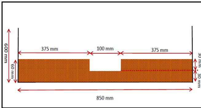
Fig. 1: The cross section of sand bed river meander channel.
