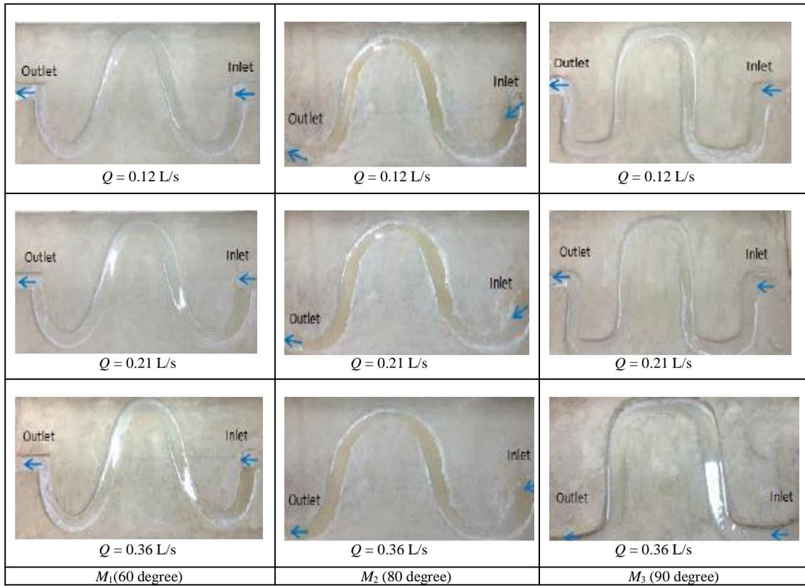
Fig.2: Meander river channel of different angle of direction  $\beta$  and flow rate  $Q$
