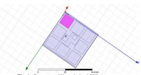
Fig. 1: Geometry of Unoptimized 3X3 Array.
