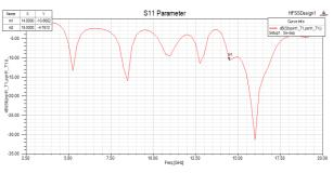
Fig. 7: Impedence Bandwidth Plot of Optimized 3X3 Array.
