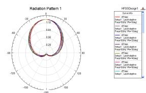
Fig. 5: Radiation Pattern of Unoptimized 3X3 Array.
