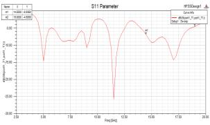
Fig. 4: Impedence Bandwidth Plot of Unoptimized 3X3 Array.
