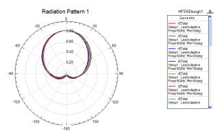
Fig. 8: Radiation Pattern of Optimized 3X3 Array.
