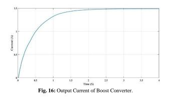
Fig. 15 and Fig. 16 shows the output voltage and current wave forms of the boost converter.
