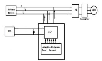
Fig. 1: Schematic Diagram of System with Distributed Generation Integration to Grid.
