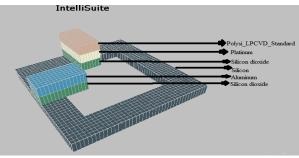
Fig. 1: Integrated Temperature and Humidity Sensor.
