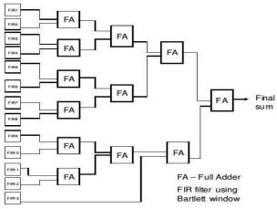
Fig. 4: Architecture of Mel Filter Bank.
