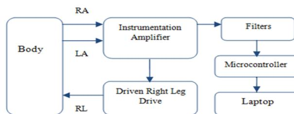
Fig. 2: Three Lead ECG Recording System.
