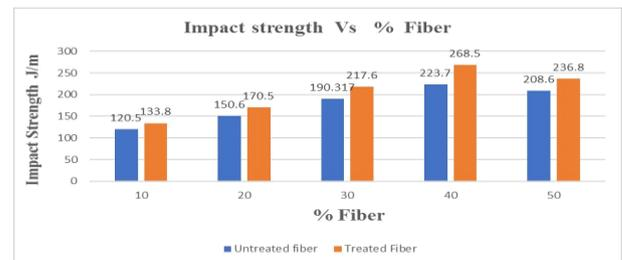
Fig. 3: Reveals the Change in the Values of Impact Strength of Unprocessed and Surface Modified Composites with the Variation of Amount of Fibers Content.
