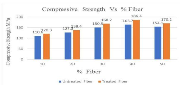
Fig. 1: Indicates The Variation of Compressive Property with Quantity of Untreated and Treated Fibers.
