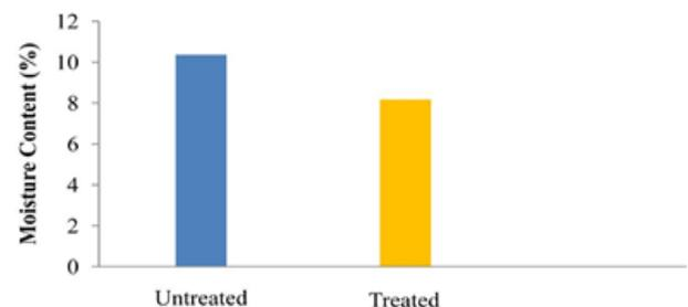
Fig. 4: Indicates the Absorption of Moisture Content by Unprocessed and Surface Modified Composites.
