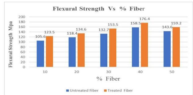
Fig. 2: Reveals The Change of Flexural Property of Unprocessed and Treated Composites with the Variation percentage of Fibers Content.
