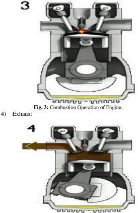
Fig. 4: Exhaust Operation of Engine.
