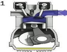
Fig. 1: Intake Operation of Engine.
