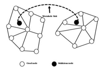
Fig. 1: Generalized Diagram of Wormhole Attack.
