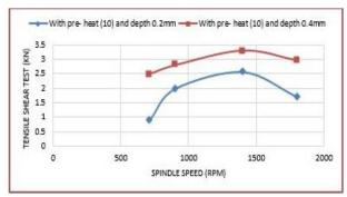
Fig. 11: Illustration Effect at Different Depth and Pre-Heat (10) Second on Tensile Shear Load.
