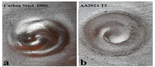
Fig. 15: Failure Mode: A) Interfacial Fracture of Carbon Steel -1006 Sheet B) Pull-Out Fracture of AA2024-T3 Sheet.
