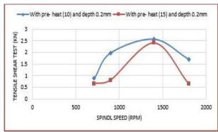
**Fig. 14:** Effect of Spindle Speed (Rpm) on the Tensile Shear Load at 0.2mm Depth of Tool with Different Dwell Time.
