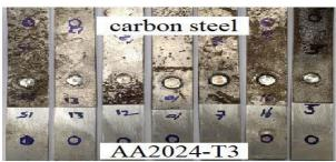
Fig.8: Samples of Welded Specimens.
