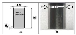
Fig. 6: Tool Geometrical Dimension, A) Tool Geometry B) Tool Photograph All Dimensions in Mm.
