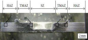
Fig. 2: Picture of Micrograph for the Cross Section of (FSSW) [6].
