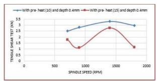
**Fig. 13:** Effect of Spindle Speed (Rpm) on the Tensile Shear Load at 0.4mm Depth of Tool with Different Dwell Time.
