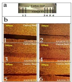
**Fig. 10:** Microstructures of the Cross-Section of Friction Stir Spot Welds for Different Regions at Spindle Speed (1400 Rpm), Feed Rate (16mm/Min), Depth of Tool (0.4mm) And Dwell Time (10sec): A) Cross Section of Weld Zone, B) Magnified Views of the Regions Respectively.
