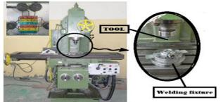
Fig. 5: Vertical Milling Machine Used to Achieve the Spot Welding.
