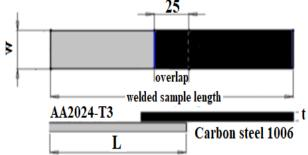
Fig. 4: Overlapping of FSSW Sample All Dimensions in Mm.
