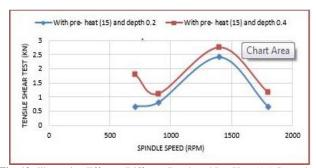
Fig. 12: Illustration Effect at Different Depth and Pre-Heat (15) Second on Tensile Shear Load.
