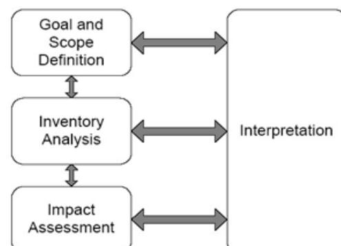
Fig. 3: An Illustration of LCA Process. (Source: Eco-Efficiency-Action-Project.Com).
