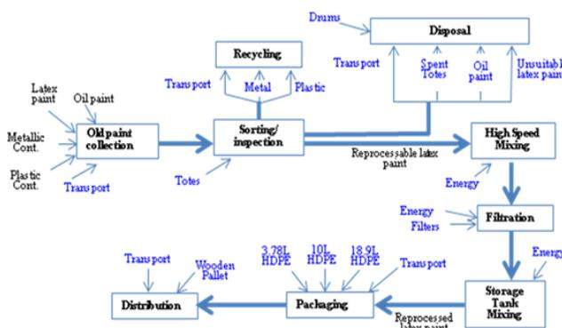
Fig. 4: The System Diagram of Recycled Latex Paint Lifecycle.
