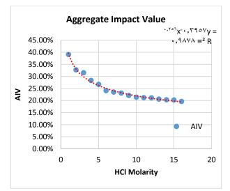
Fig. 28: The Relationship between the HCL Molarity and the Aggregate Impact Value.
