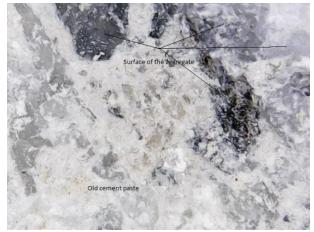
Fig. 14: The Microstructure Surface of the Treated CCWA with HCL of 1.0 Ml.
