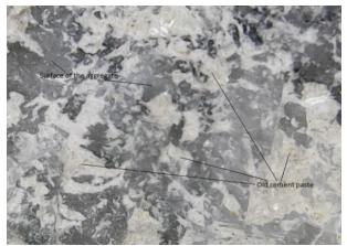
Fig. 22: The Microstructure Surface of the Treated CCWA with HCl of 9.0 ML.
