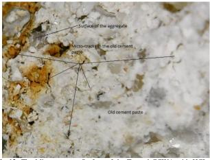
Fig 12: The Microstructure Surface of the Treated CCWA with HCL of 0.02 Ml.
