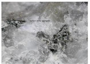
Fig. 25: The Microstructure Surface of the Treated CCWA with HCL of 12.8 Ml.
