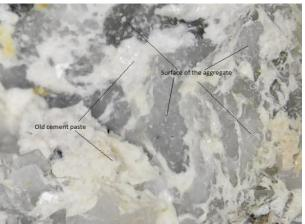
Fig. 21: The Microstructure Surface of the Treated CCWA with HCL of 8.0 Ml.
