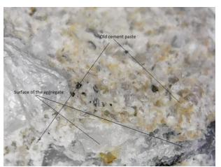
Fig. 16: The Microstructure Surface of the Treated CCWA with HCL of 3.0 Ml.
