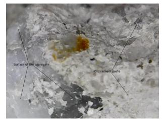
Fig. 19: The Microstructure Surface of the Treated CCWA with HCL of 6.0 Ml.
