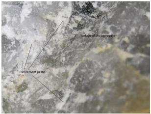
Fig. 23: The Microstructure Surface of the Treated CCWA with HCL of 10.0 Ml.
