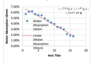
Fig. 30: The Relationship between the HCL Molarity and the Water Absorption 10 MM.
