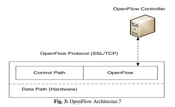
In OpenFlow architecture, datapath flow forwarding still resides on the switch, but flow forwarding decisions are made in a separate OpenFlow controller or hierarchy of controllers, which is implemented in a serv-er(s) that communicates with an Open-Flow-enabled switch(es) in the network through OpenFlow protocol.
