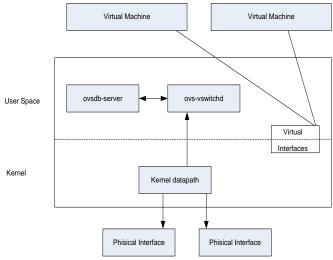
Fig. 4: Architecture of the Open vSwitch
