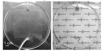
Fig. 2: The transparent fluid-filled microtubes run through the window without affecting the clarity of visibility, reproduced from Hatton et al. (2013).
