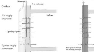
Fig. 3: Bio-inspired envelop design for heat retention in cold climate, reproduced from Badranah (2012).
