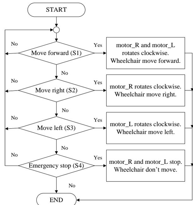
Fig. 4: Diagram of Function of Disabled Person Wheelchair.
