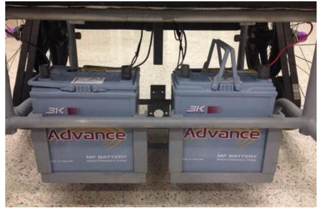
Fig. 12: Battery Used in Test.
