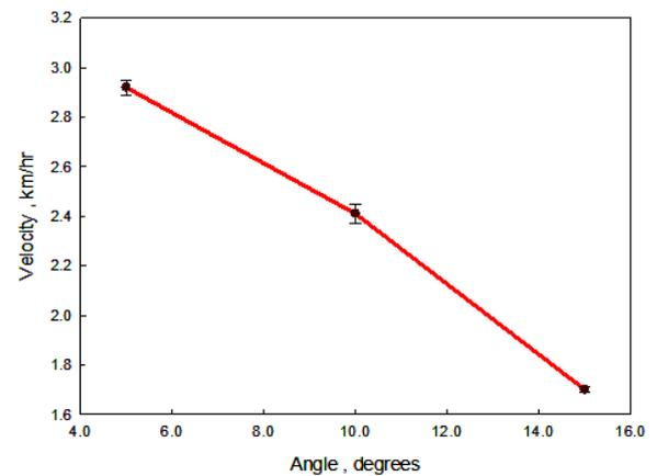
Fig. 8: Graph of Relationship between Velocity and Slope.
