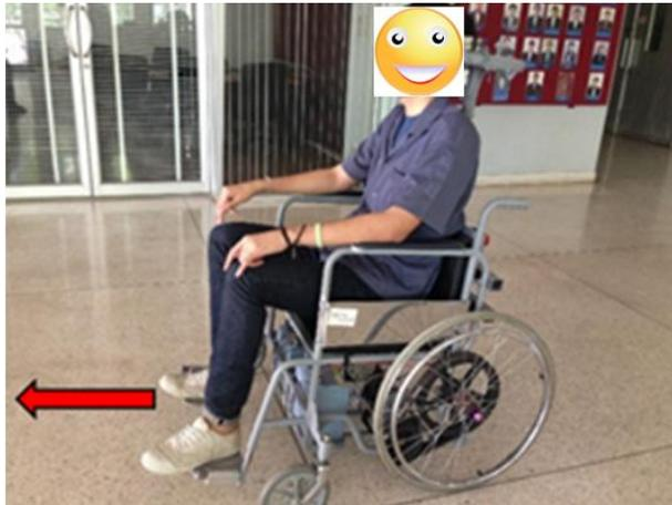
Fig. 5: Horizontal Mobility Test.
