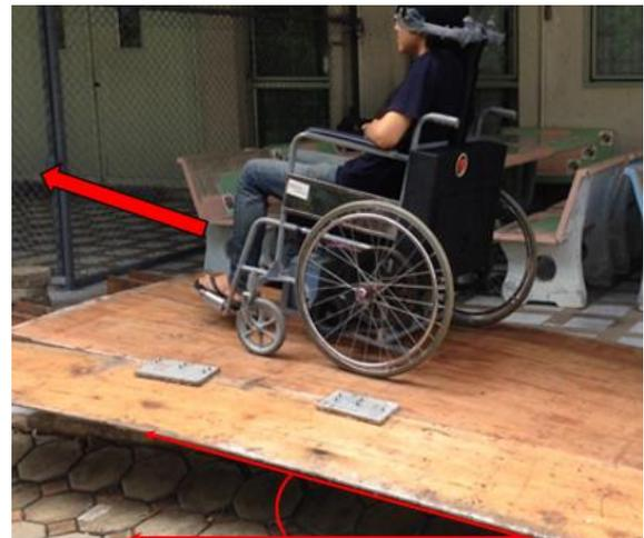
Fig. 7: Slope Mobility Test.
