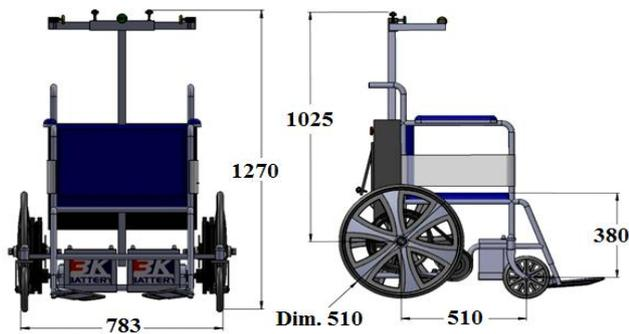
Fig. 2: Overall Size of Disabled Person Wheelchair (Unit: mm)
