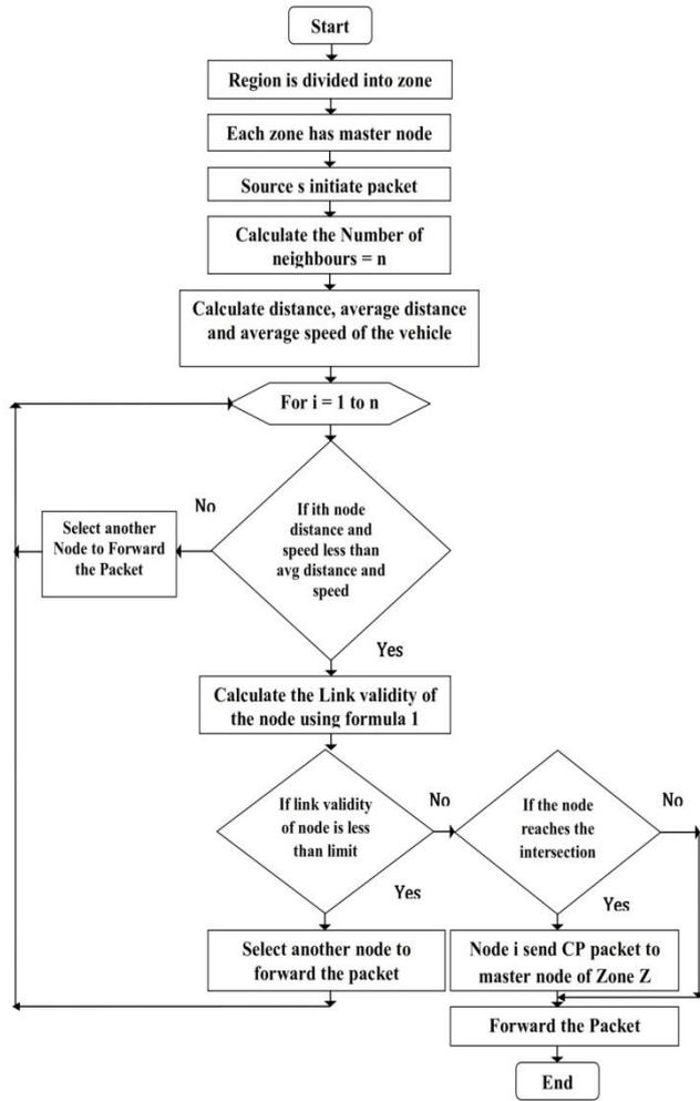
Fig. 1: Flow Chart of Geographical Zone Based Routing for Sparse Networks.
