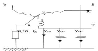
Fig. 9: The System is in A State of Disturbance on Phase T to Ground.
