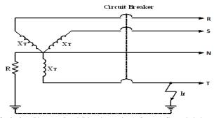
Fig.6: One Phase to Land Disturbance in A System Grounded through Prisoners.
