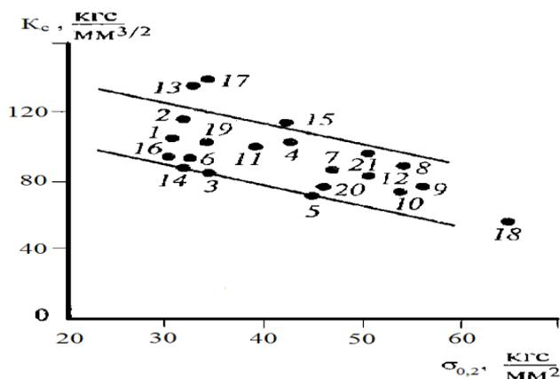
Fig. 5: Aluminum Alloys Crack Resistance Characteristics Dependence on Strength.
