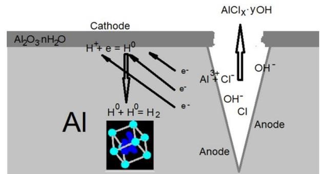
Fig. 3: Hydration Mechanism of Aluminum Alloy Corrosion in Chloride Ions Presence.
