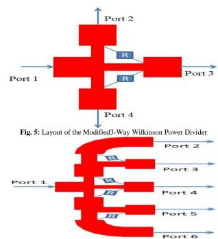
Fig. 6: Layout of the Unequal 5-Way Wilkinson Power Divider.
