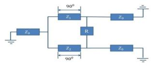
Fig. 1: Schematic Model for Wilkinson Power Divider.
