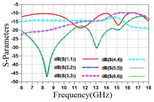
Fig. 7: Return Loss of the Proposed Design.
