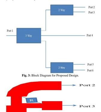
Fig. 4: Layout of the Modified 2-Way Wilkinson Power Divider
