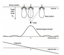
Fig 1: Doppler frequency of the target
