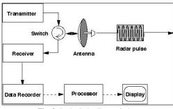
Fig. 3: Radar Pulse Transmission.
