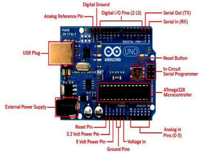
Fig. 3: Arduino UNO Board Sources: <https://www.Arduino.Cc>.
