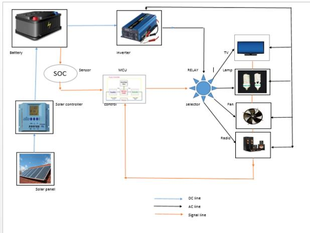
Fig. 4: Block Diagram of the SOC, Current and Power Measurement.
