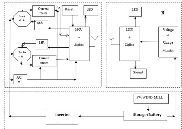
Fig. 1: Block Diagram of the Intelligent Load Management (ILM).
