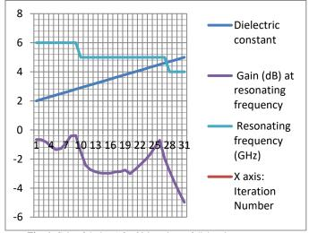
Fig. 6: Gain of design 1 for 30 iterations of dielectric constant.
