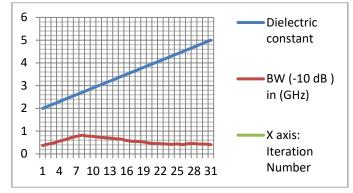
Fig. 5: Bandwidth of design 1 for 30 Iterations of dielectric constant.
