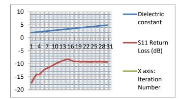
Fig. 7:.S<sub>11</sub> of design 2 for 30 iterations of dielectric constant.
