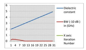
Fig. 8: Bandwidth of design 2 for 30 iterations of dielectric constant.
