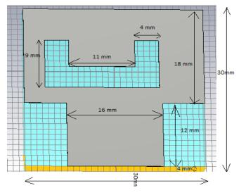
Fig. 3: U Shape Patch Antenna with thickness of 4mm.
