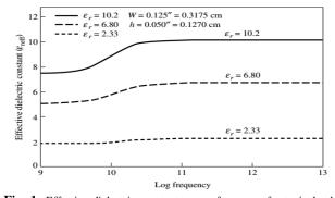
Fig. 1: Effective dielectric constant versus frequency for typical substrates.
