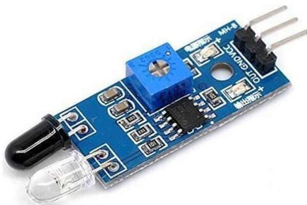
Fig. 12: Infrared Sensor.
