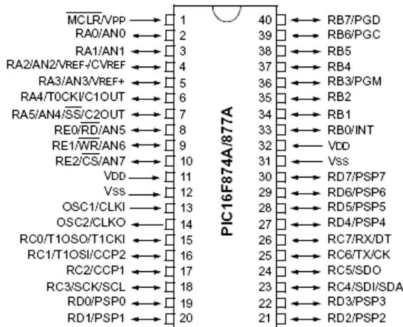
Fig. 6: Pin Diagram of PIC16F877A.
