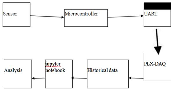
Fig. 5: Block Diagram.
