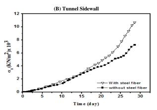
Fig. 13: Effect of Steel Fibre Content on the Development of Lining Stress with Time.
