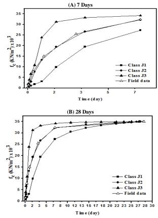
**Fig. 8:** Evaluation of Shotcrete Strength Classes with Time for A) 7 Days, B) 28 Days.
