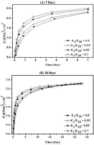
Fig. 9: Shotcrete Elastic Stiffness with Time in A) 7 Days, B) 28 Days.
