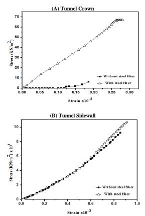
Fig. 14: Stress-Strain Curve of the Reinforced and Unreinforced Tunnel Lining.
