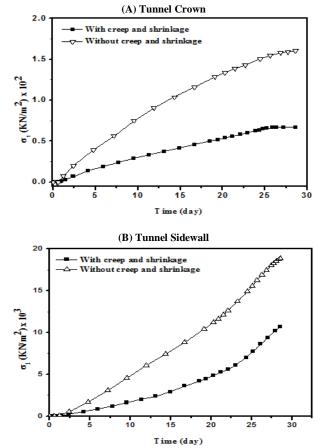
Fig. 10: Effect of Creep and Shrinkage Strain on Development of Shotcrete Stress with Time.
