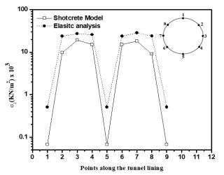
Fig. 17: Major Principal Stress along the Tunnel Lining Using the Shotcrete Model and the Elastic Analysis.
