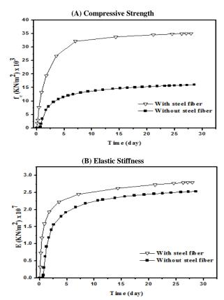
Fig. 12: Development of Compressive Strength and Elastic Stiffness of Reinforced and Unreinforced Tunnel Lining with Time.
