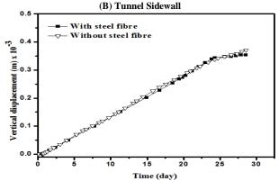
Fig. 15: Effect of Steel Fibre Content on the Development of Lining Displacement with Time.
