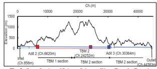
Fig. 3: Cross Section of Pahang-Selangor Water Transfer Tunnel.
