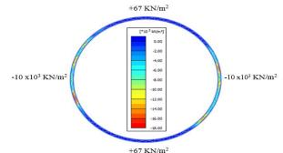
Fig. 6: Principal Compression and Tensile Stresses along the Tunnel Lining.
