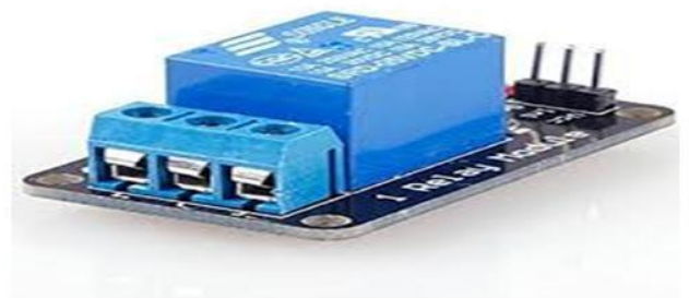
Fig. 3: Relay for switching
