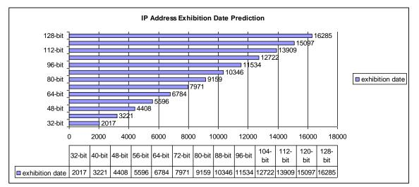
Fig. 4: prediction of exhaustion date for the available address space for an IP address range from 32-bit to 128-bit. To cover the range from 32-bit to 128-bit, we picked an interval of 8 bits length between two consecutive addresses size.(ex: exhaustion date for 32-bit address is 2017)
