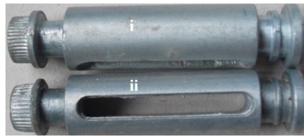
Fig. 2: Photographs of Non-Plated (I) as Received and (II) Cast Al Alloy Pistons.
