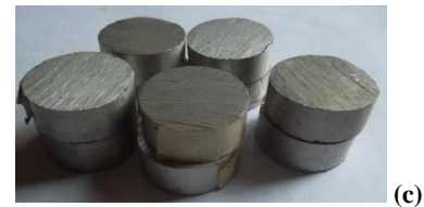
Fig. 1: (a) Sketch diagrams, photographs of (b) piston specimens and (c) coupon for corrosion tests
