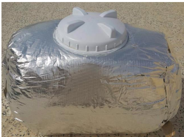
Fig. 1: Overhead Water Storage Tank with Insulation (Case 2).
