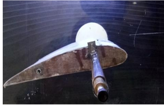
Fig. 11: Side View of the Stream Lines over Wing at 15 Degree AoA.
