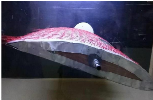
Fig. 8: Side View of the Tufted Airfoil in Wind Tunnel at 15 Degree AoA.
