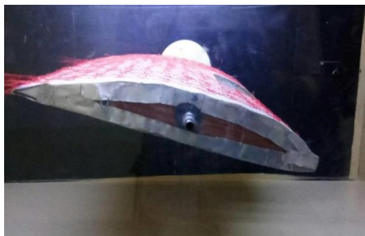
Fig. 9: Side View of the Tufted Airfoil in Wind Tunnel at 25 Degree AoA.
