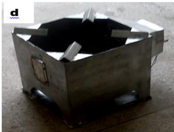
Fig. 1: C) Wind Chamber of the Cook Stove.
