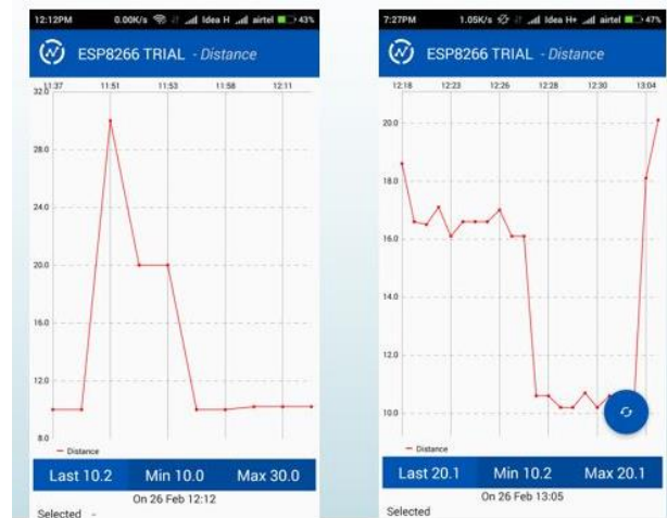
Fig. 7: Sample Data Uploaded on Cloud Server and Results from Things View App.
