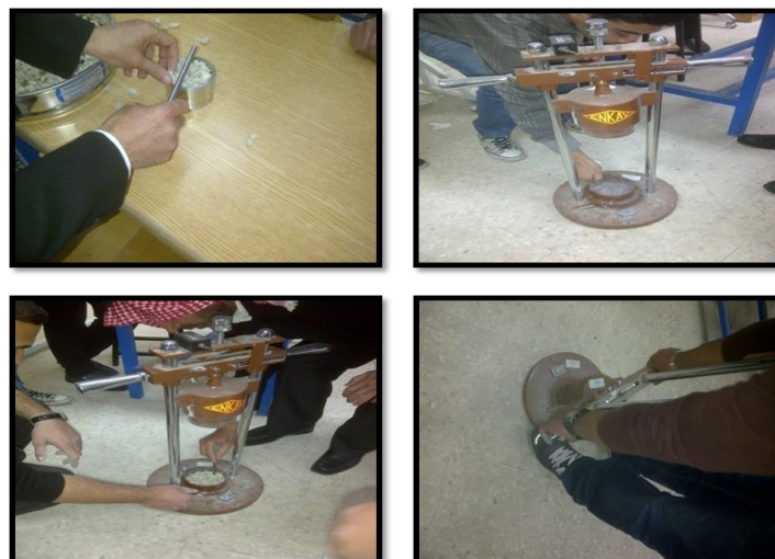
Fig. 3: Test Procedure for Aggregate Impact Value.
