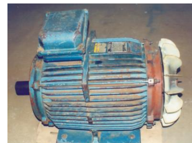
Fig. 1: (C): Motor As Re-Assembled And Made Ready For Workshop Test-Running.
