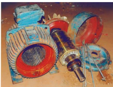
Fig. 1: (A): Motor As Dismantled And Made Ready For Physical Measurement & Inspection.
