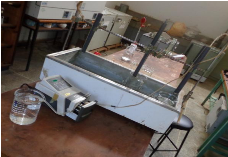
Fig. 3: Experimental Photo of the Mini Column Continuous Fluoride Adsorption onto Crushed Burnt Clay Pot
