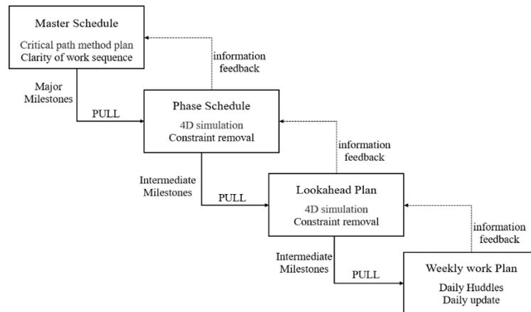
Fig. 1: The Application of LPS with BIM.
