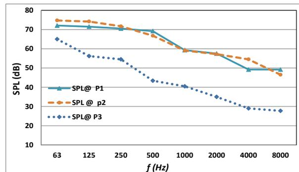
Fig. 1: Results of Measured Octave Band Sound Pressure Levels at Positions 1, 2, 3.
