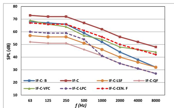
Fig. 6: A) Calculated Outdoor Sound Pressure Levels with Different Noise Reduction Methods.
