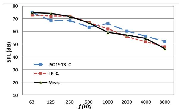
Fig. 3: Comparisons Between the Measured and Calculated Sound Pressure Levels at Position 2.
