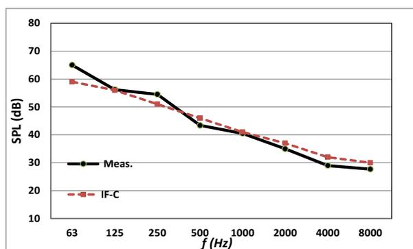
Fig. 4: Comparison Between the Measured and Predicted Sound Pressure Level Values at Location 3.
