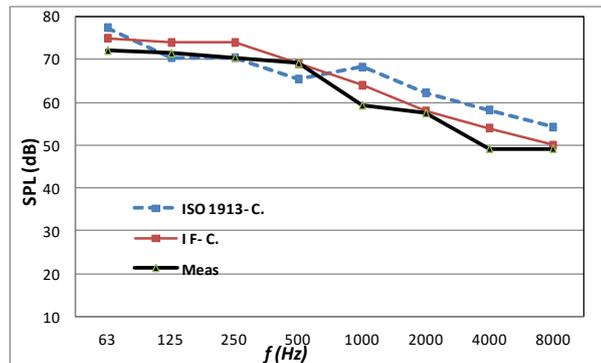
Fig. 2: Comparison between Measured and Calculated Octave Sound Levels at Position 1.
