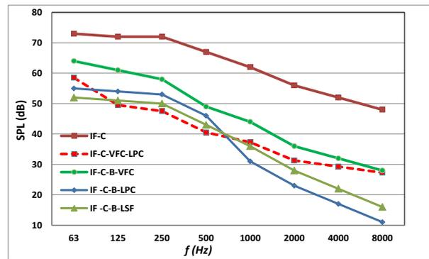
Fig. 6: B) Calculated Outdoor Sound Pressure Levels with Different Assembly Noise Reduction Methods.
