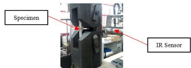
Fig. 1: The IR sensor and the specimen set up
