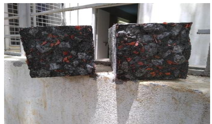
Fig. 10: Flexural Failure Of Specimen At 28 Days
