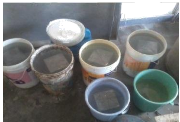
Figure 4.3: curing of cubes in chloride solution
