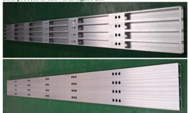
Fig. 17: Aluminum plate top and bottom view after complete process
