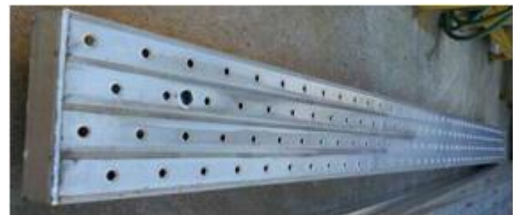
Fig. 2: Previously used iron plate scaffolding board
