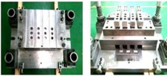
Fig. 9: Assemble of die upper and lower body
