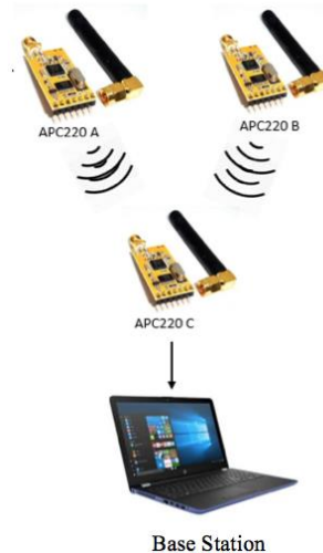
Fig. 2: Wireless Sensor Network Topology Using APC220
