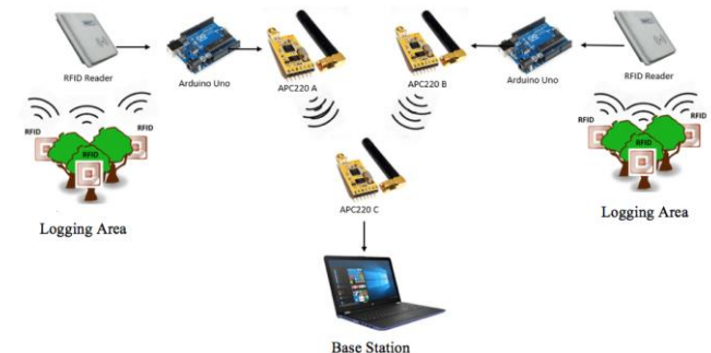
Fig. 3: Illegal Logging Tracking Proposed System
