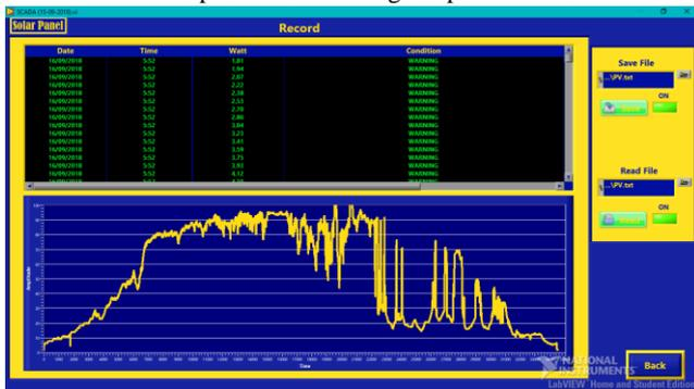
Fig. 10: Result of HMI test on PV section
