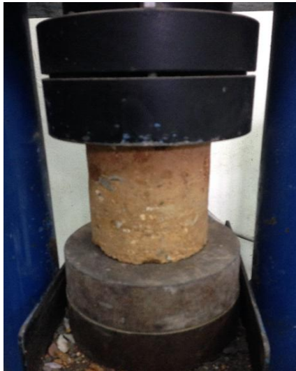
Fig. 3: Compression Test on Extracted Sample.
