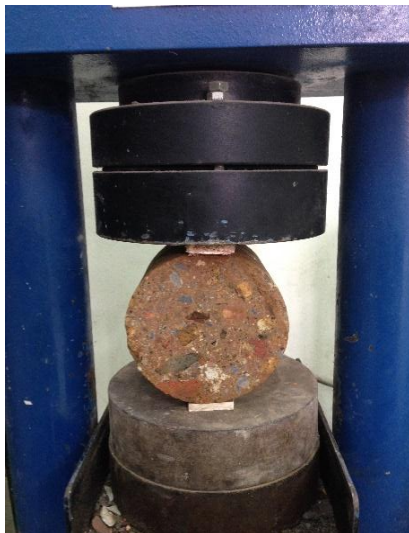
Fig. 4: Splitting Tensile Test on Extracted Sample.
