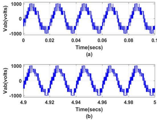
Fig. 13: Line Voltage with Proposed PWM Technique with UPF Load
