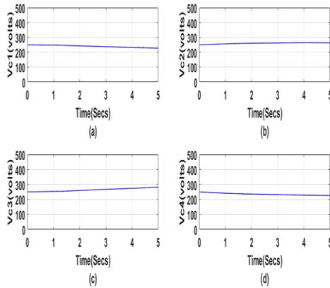
Fig. 12: Capacitor Voltages with Proposed PWM Technique with UPF
