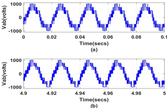
Fig. 15: Line Voltage with Proposed PWM Technique with 0.2 Lag Load
