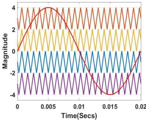
**Fig. 2:** Reference and Carrier Signals for Conventional CBPWM
