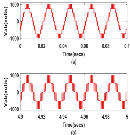
Fig. 11: Line Voltage with Conventional CBPWM Tech. with 0.2 Lag Load
