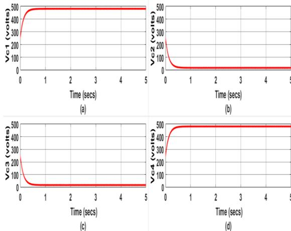
Fig. 8: Capacitor Voltages with Conventional CBPWM Tech. with UPF Load
