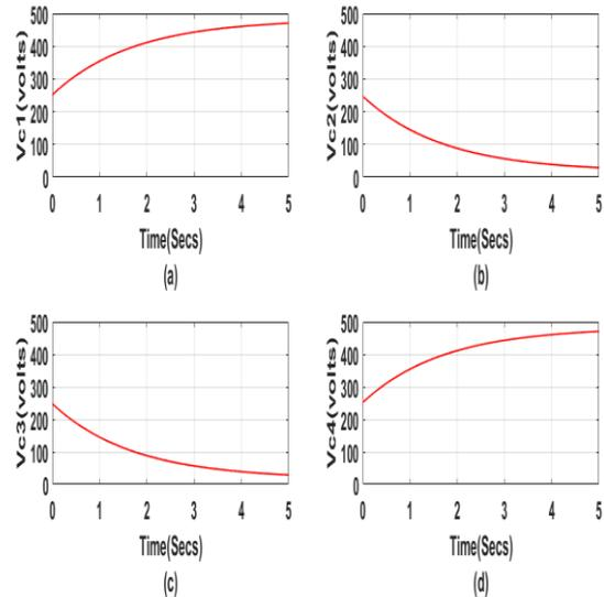
Fig. 10: Capacitor Voltages with Conventional CBPWM Tech. with 0.2 Lag Load
