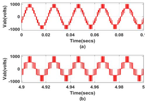
Fig. 9: Line Voltage with Conventional CBPWM Tech. with UPF Load
