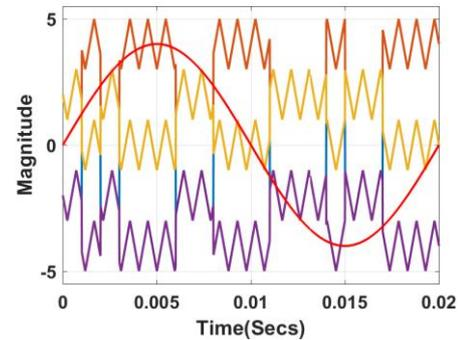
Fig. 6: Reference and Carrier Signals for Proposed PWM Technique.
