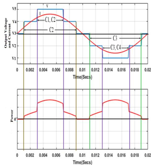
**Fig. 3:** Effect of switching on Capacitor Voltage imbalance for UPF Load
