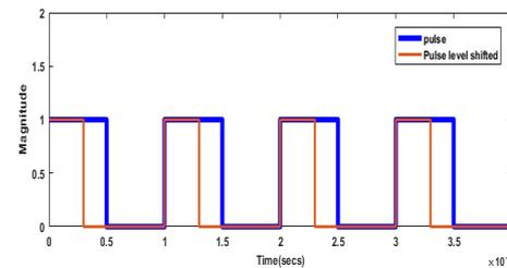
Fig. 7: Variation in pulse width due to added DC Off- set
