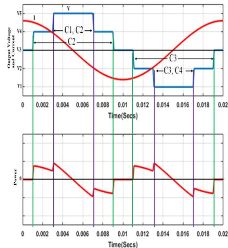
**Fig. 4:** Effect of switching on Capacitor Voltage imbalance for ZPF Load
