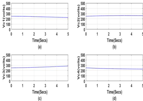
Fig. 14: Capacitor Voltages with Proposed PWM Tech. with 0.2 Lag Load
