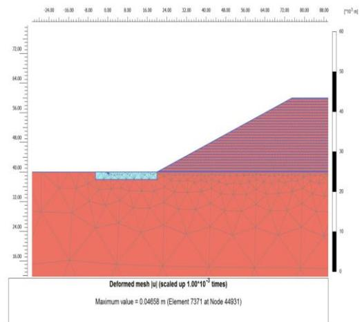
Fig. 5: Filling of 2m foundation pit with reinforced soil
