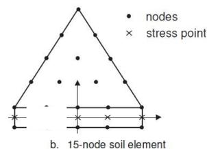
Fig.2: Nodes and stress points distribution of interface elements and their connection to soil elements
