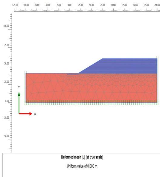
Fig. 3: The existing ground of initial phase in staged construction mode
