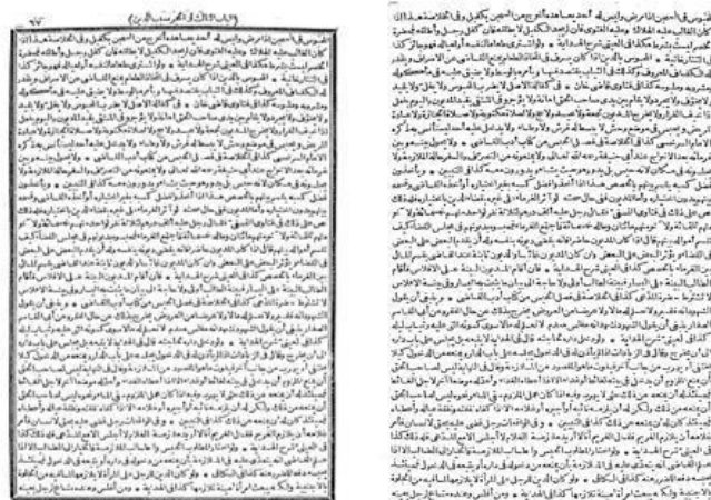
(a) Before frame removal (b) After frame removal Fig. 6: Frame detection and removing for Arabic document
