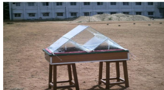
Fig. 1: Photograph of double slope multi sponge liner basin solar still.
